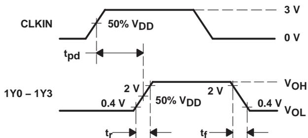
**Figure 8. Voltage Threshold for Measurements, Propagation Delay ( $t_{pd}$ )**
