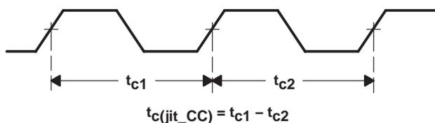
**Figure 10. Cycle-to-Cycle Jitter**
