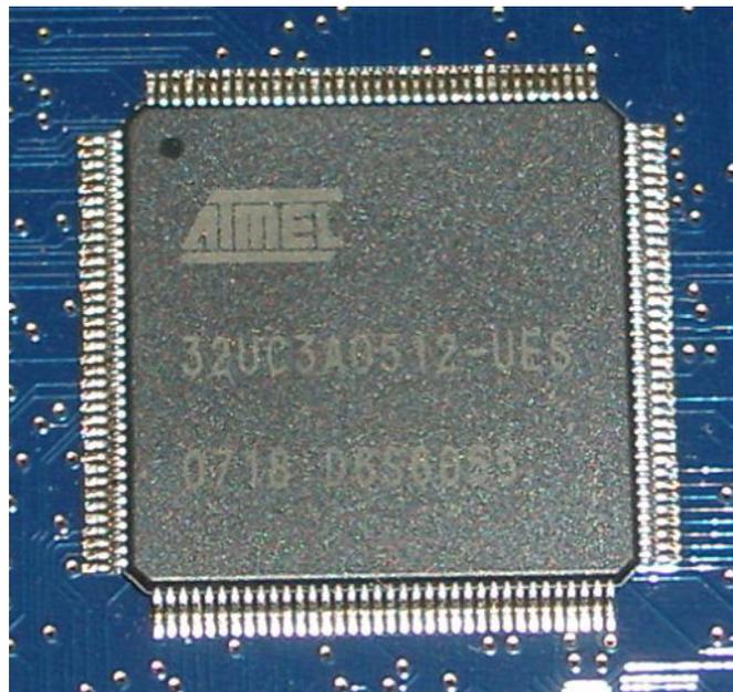
To check which type of MCU is mounted on your EVK1100 evaluation board, you can read the part number printed on the MCU. The picture shows the part number printed on an -ES part (-UES suffix).
