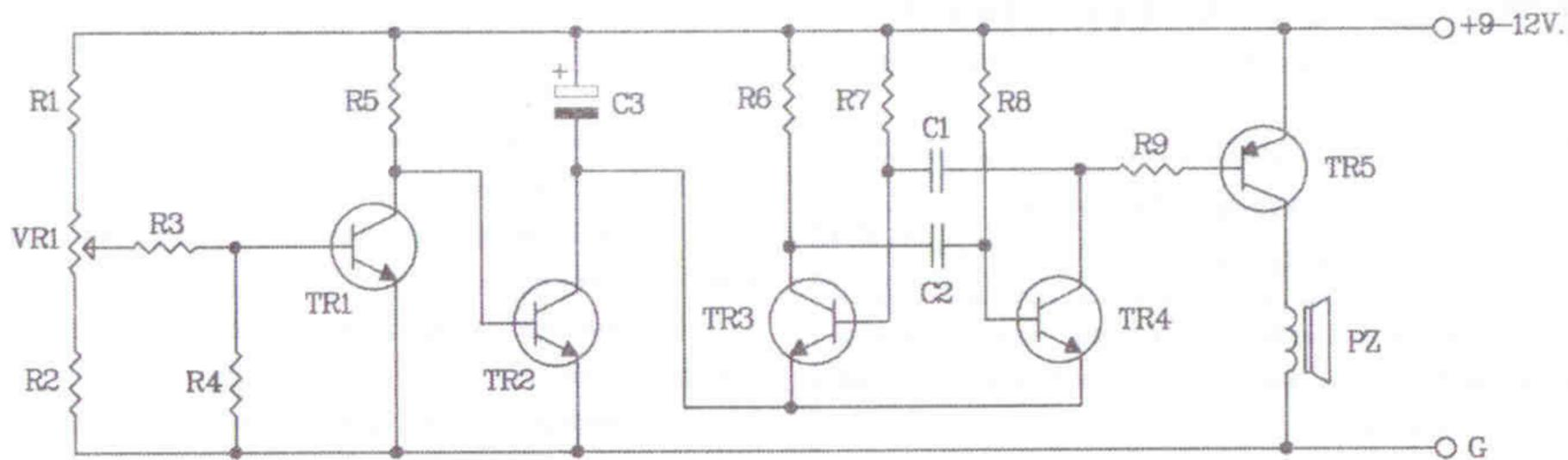
Figure 2. The low battery alarm (for 12V) circuit
