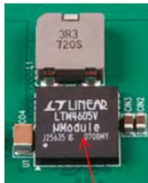
Figure 2- First uModule buck-boost regulators allowed novice system designer easy access to complicated design.
